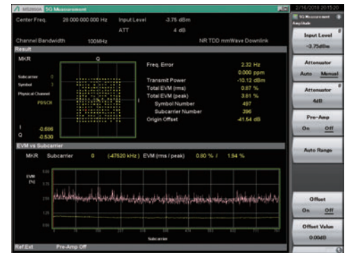
Basic MS2850A Measurement Screen (EVM vs. Subcarrier)
